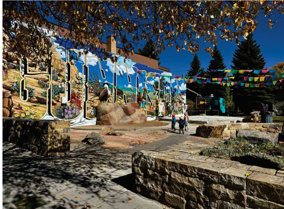
IOOF Park – All of the stone seat walls were constructed using stone that was salvaged from an old city shop building. The “shop block” became an integral part of the design as well as a catalyst for reminiscing and storytelling.
